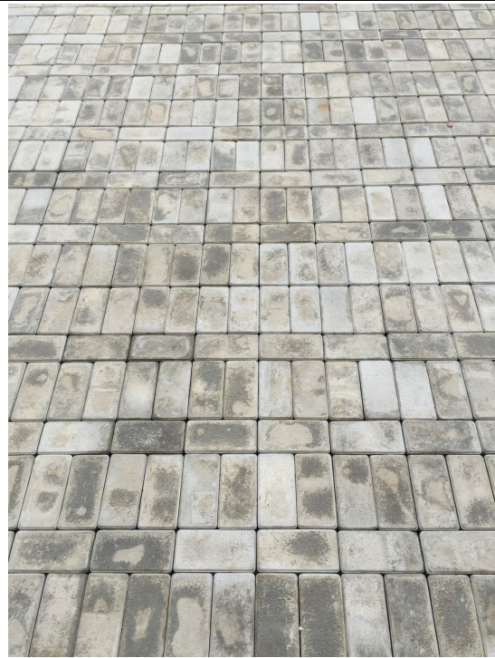
Sampling done at customer site by rubber mould . Outcome after one rain cycle
